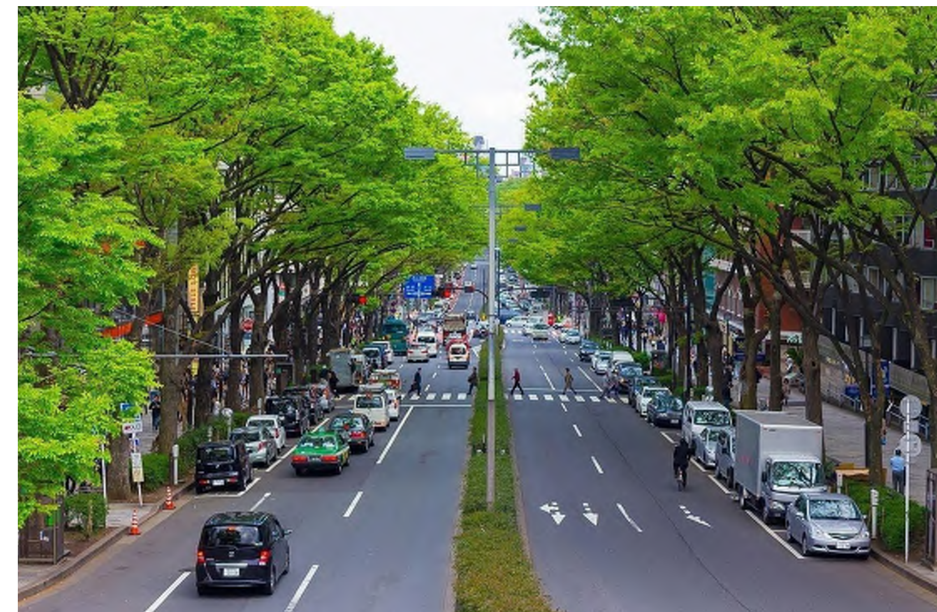
3. The use of larger, "monumental" street trees help reduce pollution, heat, and runoff while reducing visual clutter and provide traffic calming by making the road appear narrower.
