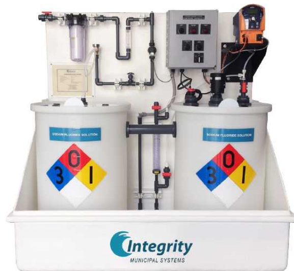
Figure 1: Typical modular upflow saturator device (image courtesy of Integrity Systems, Inc.); Granular Sodium Fluoride is added to chamber on left and softened water is passed through the granular material resulting in concentrated brine which is accumulated in tank at right, a separate metering pump (orange item) is then used to meter chemical dosage into the water system.
