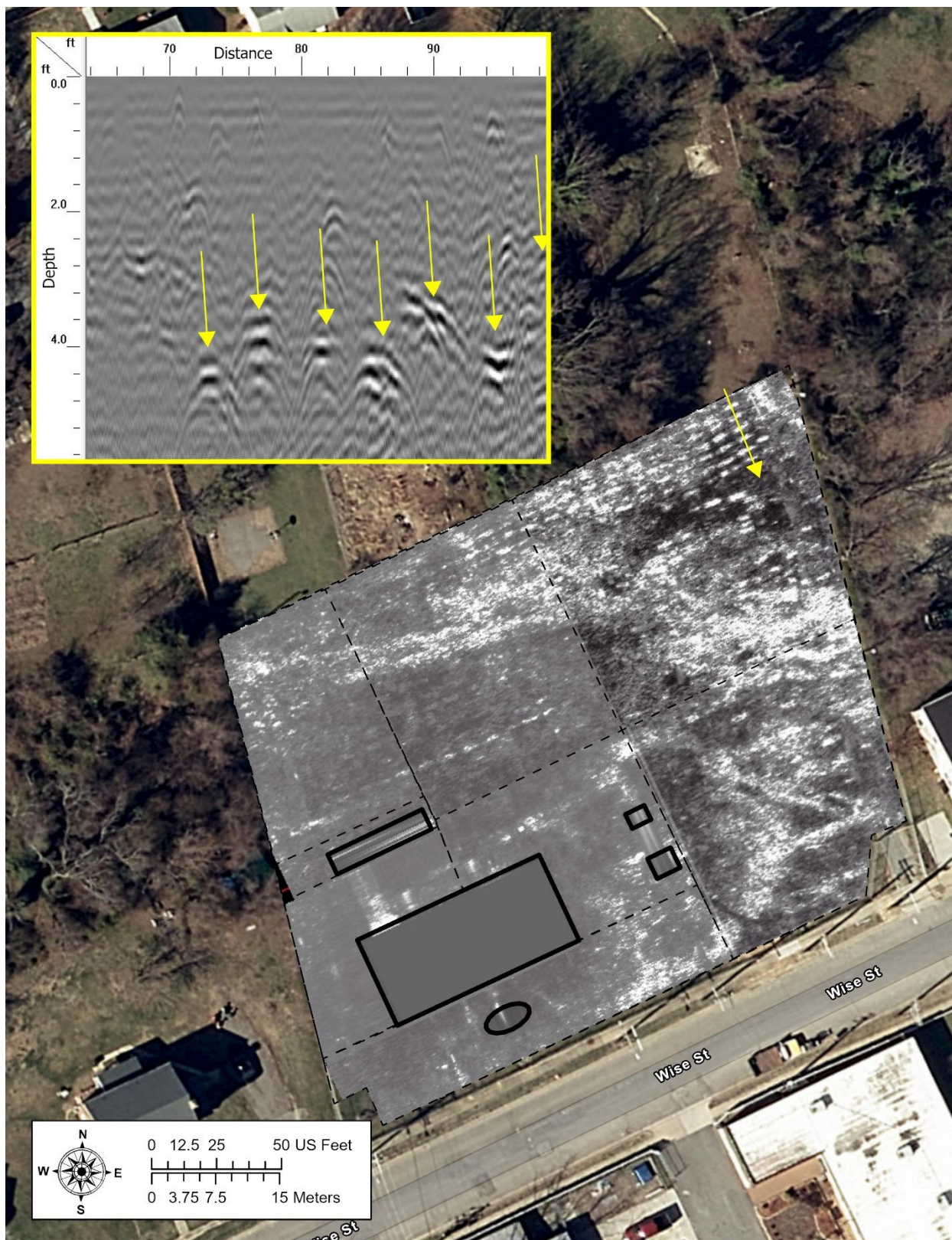
Figure 2.3. An example of a 19 th -century cemetery associated with the Weisinger-Carroll Hospital, City of Richmond, Virginia. The inset shows the high-amplitude targets representing probable coffins (yellow arrows).
