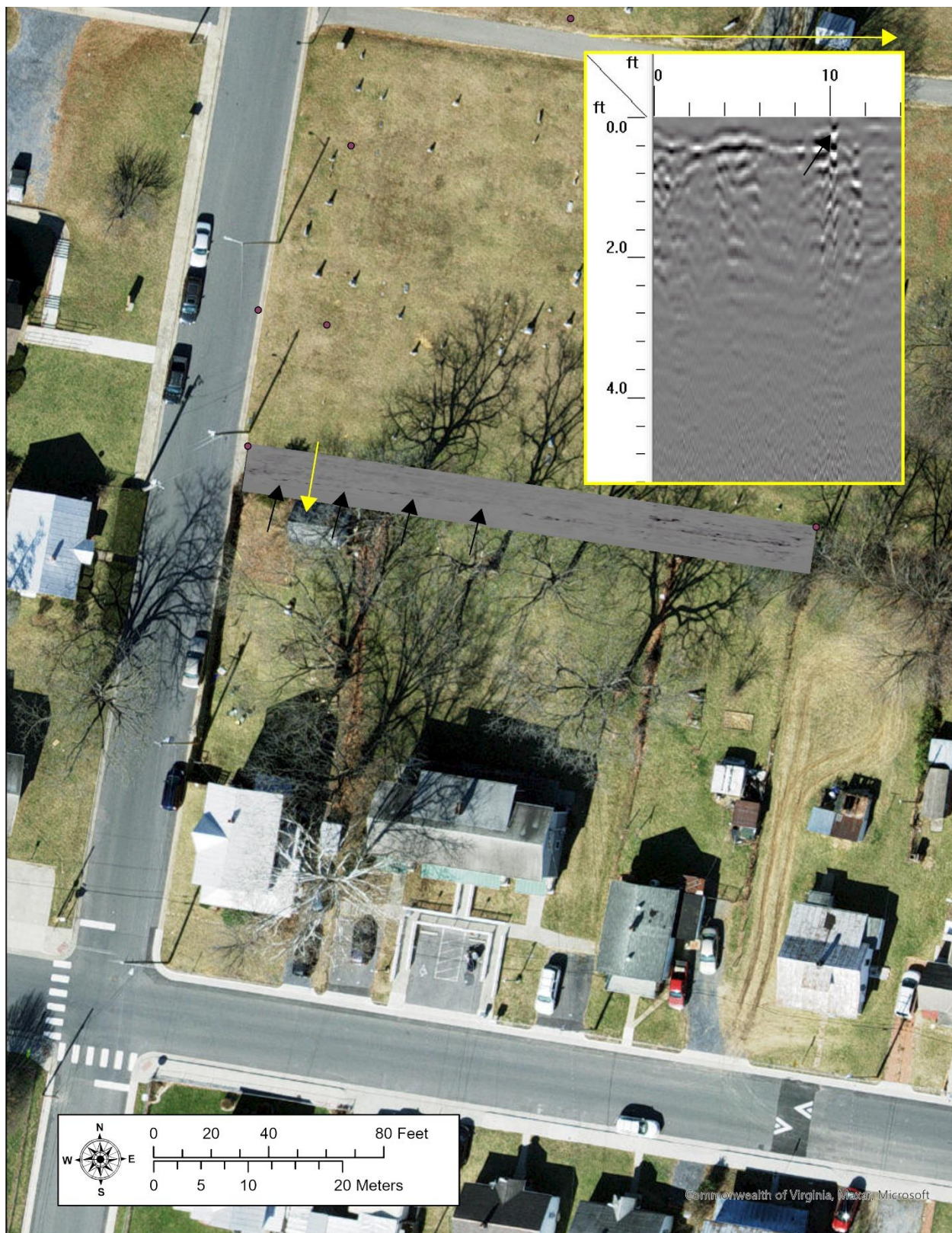
Figure 4.4. Shallow, high-amplitude linear target (black arrows) located in the alleyway gridded survey area. The profile of the feature, likely a communication line (i.e., cable, fiber, or phone), is shown in the inset (black arrow).
