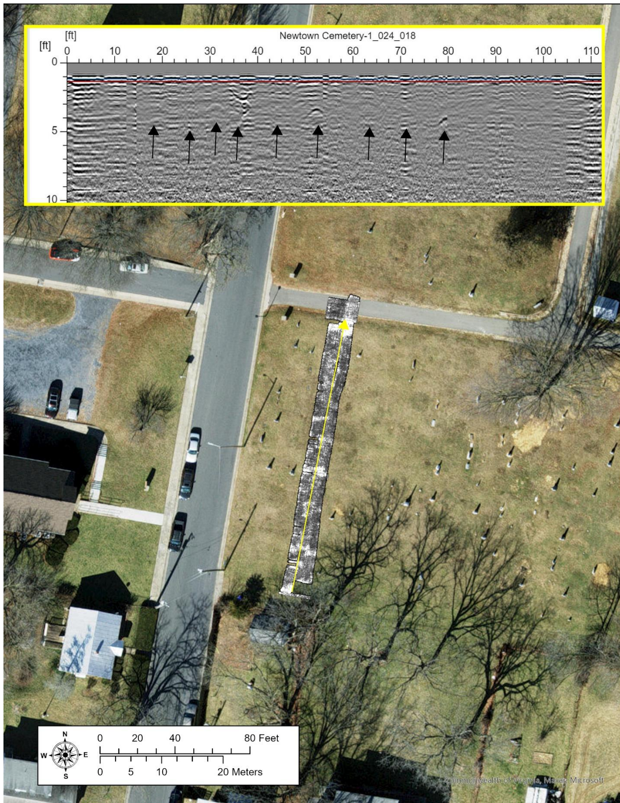
Figure 3.3. Prospection line (yellow arrow) and corresponding reflectance profile (inset) from the MALA MIRA HDR multi-channel array. The black arrows indicate probable coffins (inset).
