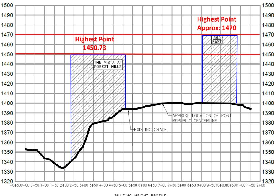
NOTE: PROFILE IS ONLY MEANT TO BE ILLUSTRATIVE OF HOW TALL THE PROPOSED PROJECT WILL BE WHEN COMPARED TO 865 EAST. PROFILE DOES NOT
