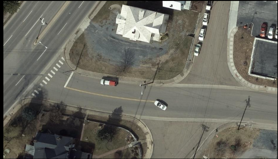
Stop bar and double yellow line at stop sign
