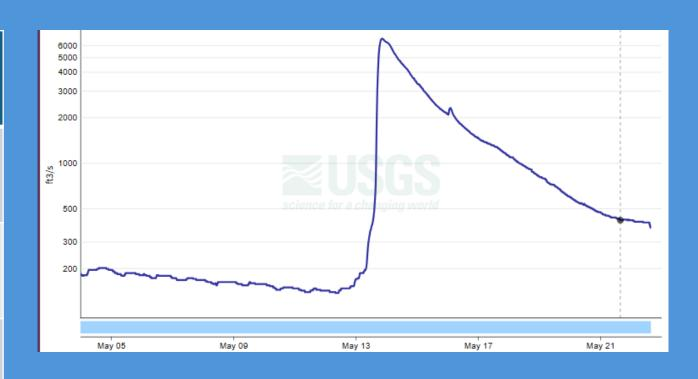
The rains of May 12 quickly moved the Harrisonburg water sources to the characteristics of rainwater runoff
