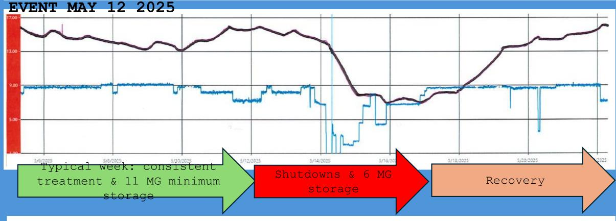
Primary Effect: Less efficient coagulation created more extensive filtration cleaning & backwash volume
